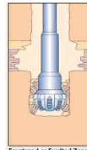
Fractured or Faulted Zone
